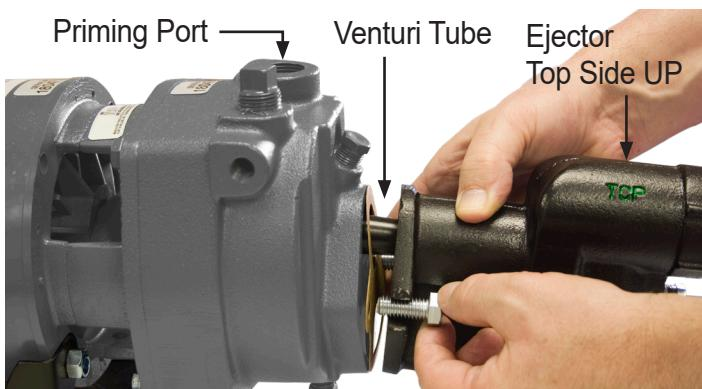
Attach ejector to face of pump with two (2) bolts and gasket provided. Venturi tube on the ejector inserts into the top tapping of the face of the pump
