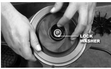
9. Once the lock washer is removed, slide the impeller off of the shaft.
