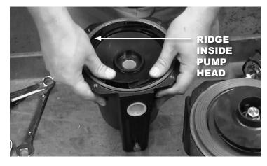
19. Reinstall the o-ring so it seats inside the ridge inside the pump body.
