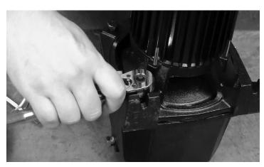
22. To reinstall the fan, find the flatted portion of the fan opening and the flatted portion of the shaft. Line those two up. Press the fan back in place and replace the motor cover.
