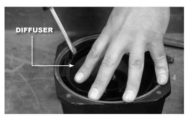
18. Discard the old diffuser, and install the new one from the repair kit. Alignment isn't required, but it may need a tap from a rubber mallet to seat back into the ridge inside the pump head.
