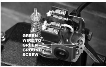
25. Replace the cover on the pressure switch to complete the repair.
