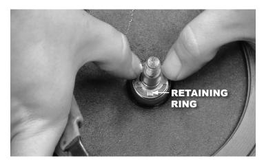
15. Replace the key in the keyway, and reinstall the impeller, keeping the slot in the impeller lined up with the key.
