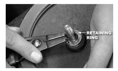
12. Remove the flat washer located under the retaining ring, and pry the seal off of the shaft with a flat screwdriver. Discard the old seal.
