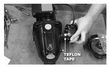
24. Insert the wires through the strain relief nut and then through the strain relief. Connect the green wire to the ground screw. The black and white leads can be connected to either inside terminal. Attach all three wires and hand-tighten the screws.
