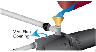
b. Slowly fill the discharge tee with water until water overflows the vent plug opening. NOTE: Before turning on pump, loosely replace vent plug and open several outlets or faucets to allow water flow during priming.
