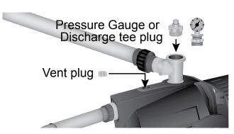
c. Check to be sure water in the cavity of pump stays constant. If water level goes down, it could indicate a leak in the foot valve, check valve, or suction pipe. If water remains constant, wrap the pressure gauge or discharge tee plug, and vent plug threads with thread tape, and thread into pump. Tighten with wrench (not included).
