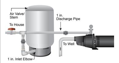
Air pressure in the tank must be 2 PSI lower than the "cut-in" of the pressure switch. Pump has a 20/40 PSI pressure switch, so tank pressure must be set at 18 PSI. Check pressure with a tire gauge (not included) and add or subtract air as needed.
