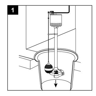
2. Connect the discharge pipe, fittings and check valve (not provided) to pump (A) discharge according to local codes. The discharge pipe should be the same size as the discharge of pump (1-1/4 in.) or larger.
