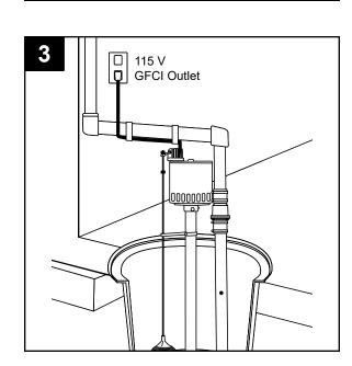
4. Test the operation of the pump by pouring water into the sump basin.
