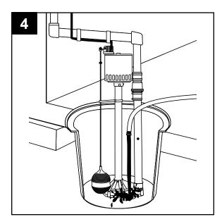
5. If the lower rod stop is positioned 8 in. from the top of the rod, the pump will turn on at approximately 10 in. to 12 in. and off at approximately 2-1/2 in. To cycle the pump on and off faster, move the lower float stop closer to the float rod guide.
