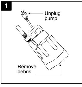
If pump clogs, unplug the pump from the power supply. Attach one end of a garden hose to a spigot and the other end to pump discharge. Turn on the spigot to run water through pump to clean it out.
