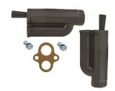
Shallow Well "SW" Ejector 2-Way Convertible "DW" Ejector For shallow or deep well installations. Includes: Ejector, gasket, and bolts for shallow well or deep well applications. (Requires 4" well casing for deep well installations).
