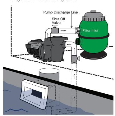
4. Connect return line from filter to swimming pool return inlet.
